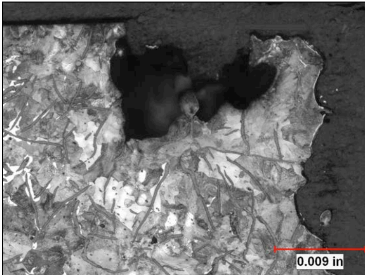
Photo 4: Mag: 100X; Etchant: 3% Nital Sample #1: Defect profile was irregular and fissure-type
