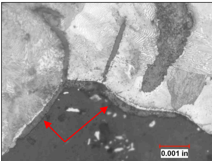
Photo 6: Mag: 500X; Etchant: 3% Nital Close-up view of inset in Photo 5 showing a layer lining the defect.
