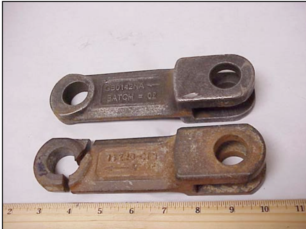
Photo 1: View of the submitted Chain samples showing fractured MCV at the bottom and 4B at top.
