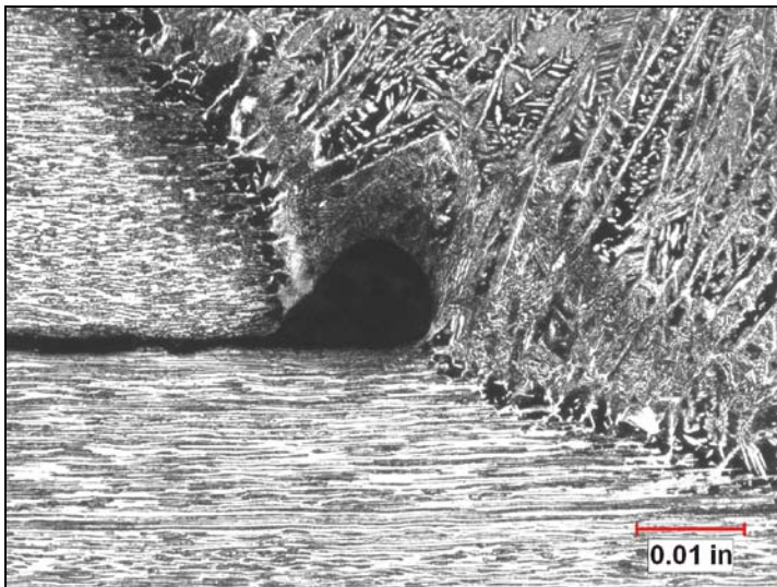
Photo 9: Mag: 50X; Etchant: Hot HCl solution Weld underfill condition (denoted with red arrow on Photo 8)
